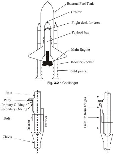
Fig. 3.2 b Field joint before ignition
